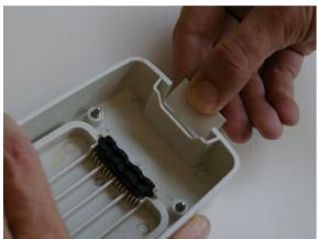
10. Now connect the cables from the turntable on the cables from the interior of the vehicle, within the casing (see illustration on the right).
